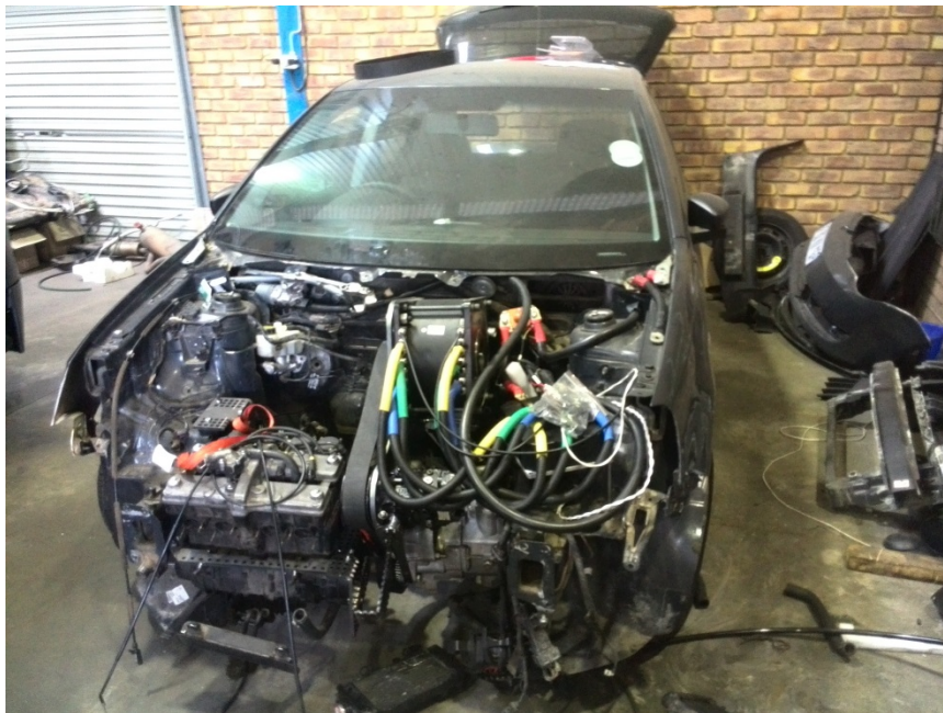
Figure 1: The modified Polo 1400 small vehicle consisting of three drivetrains.
