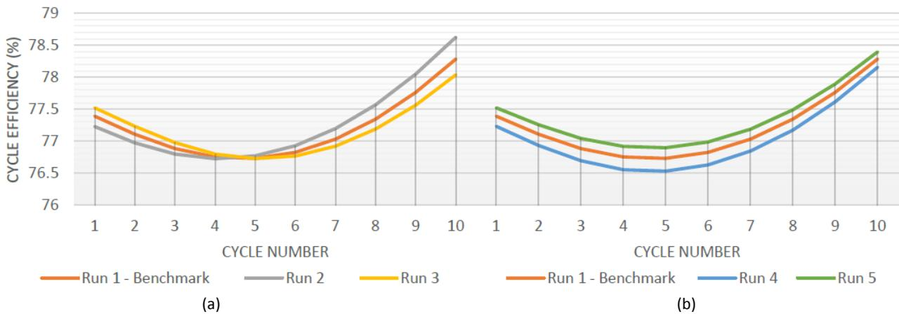
Fig. 10 Cycle efficiency as a function of (a) Maximum system pressure, (b) Flywheel inertia
