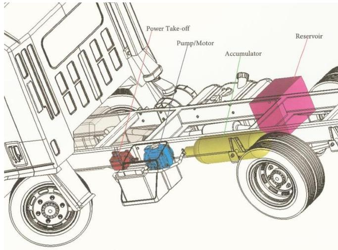
Fig. 1- MISER System layout (Adapted from Ref. [1])
