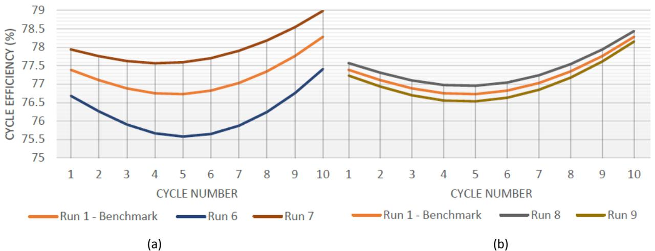
Fig. 11. Cycle efficiency as a function of (a) Nitrogen pre-charge pressure and (b) Accumulator volume
