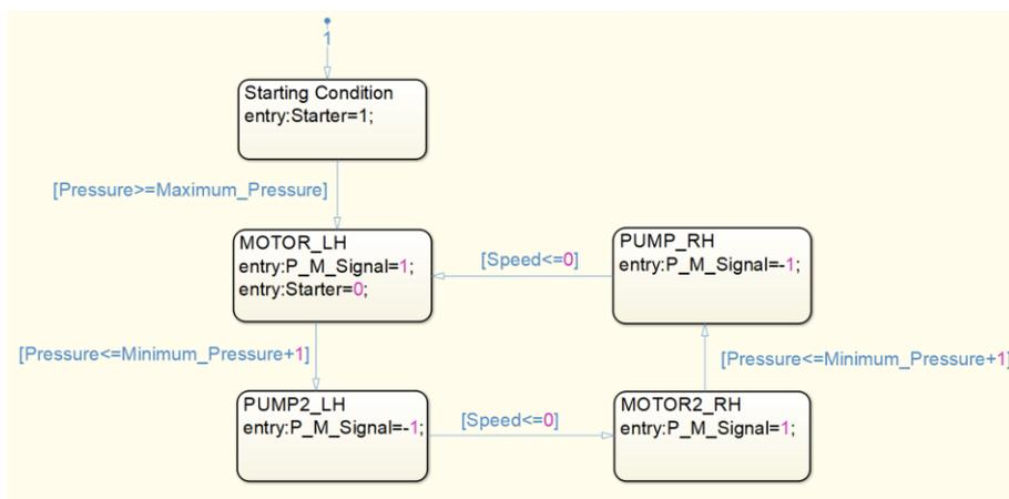
Fig. 3- State Flow Controller
